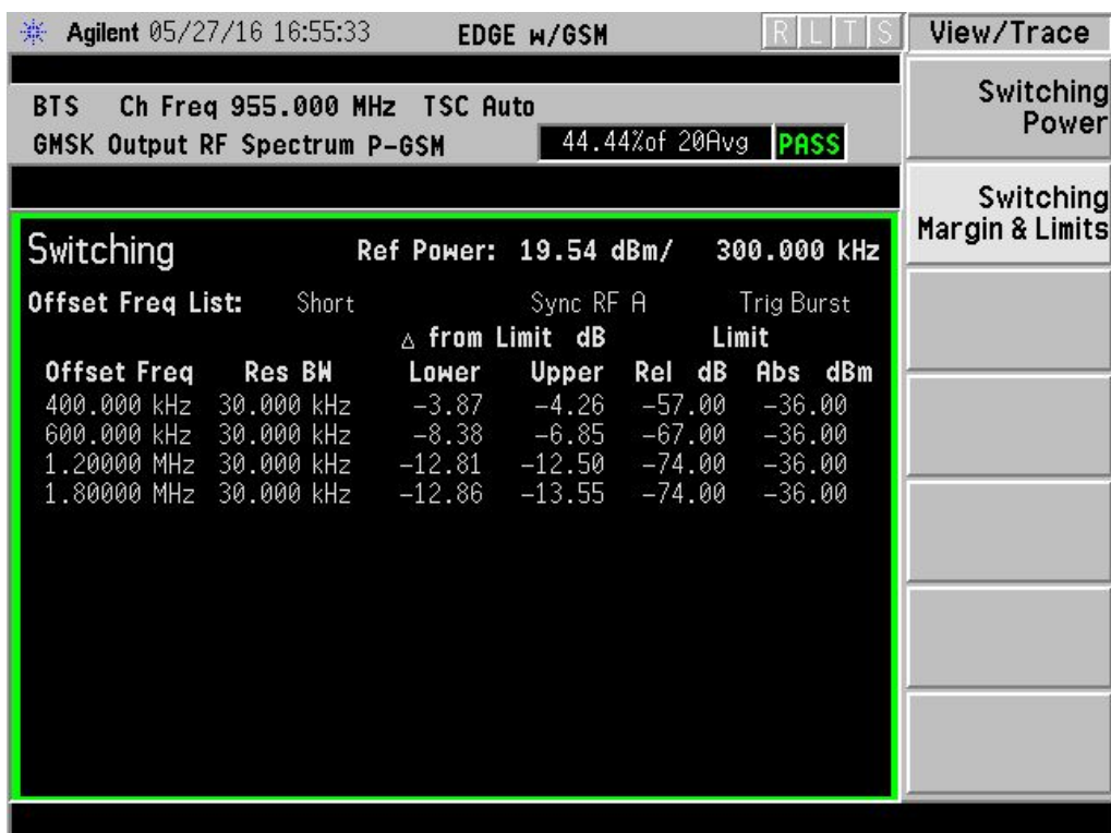
GSM-900 switching spectrum mask with osmo-trx
